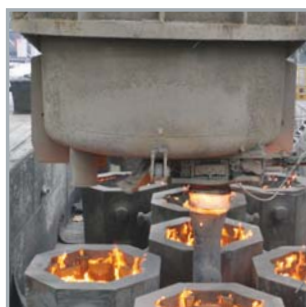
Ingot Casting (11~80tons)
